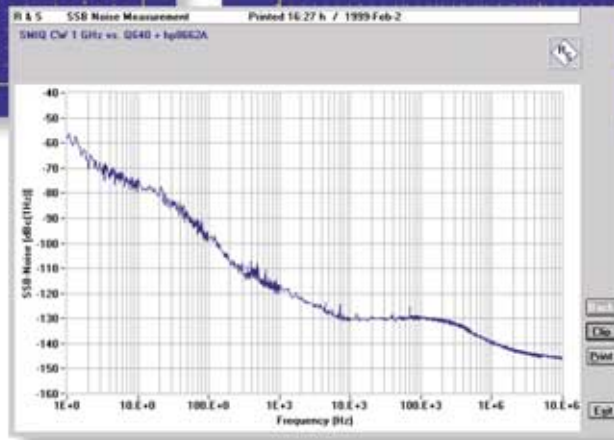
Typical SSB phase noise at f_c=1 GHz
